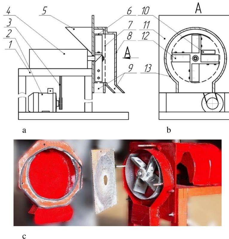
Fig. 1. **Structural arrangement of the experimental grain crusher:** a) – general view; b) – side view (the cover and the end sieve removed); c) – photo scheme: 1 – frame; 2 – electric motor; 3 – belt drive; 4 – casing; 5 – loading hopper; 6 – peripheral sieve; 7 – end sieve; 8 – housing cover; 9 – discharge nozzles; 10 – loading opening; 11 – plate; 12 – rotor with blades; 13 – housing
