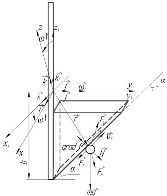
Fig. 2. Movement of grain along the blade in the crushing chamber:
